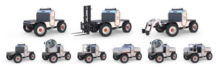
Componentized modular design with Type I, II and III hydraulic tool circuits, to accommodate over 250 CAT®, Bobcat® and John Deere® attachments
