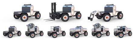
Componentized modular design with Type I, II and III hydraulic tool circuits, to accommodate over 250 CAT<sup>®</sup>, Bobcat<sup>®</sup> and John Deere<sup>®</sup> attachments
